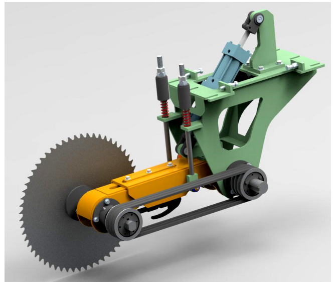
RIGHT HAND DROP SAW TRIMMER WITH MINUS 1' SAW AND EVEN ENDING IDLER ROLLS
