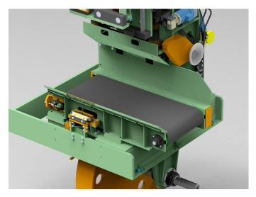
Heavy Duty offbearer constructed of 3/4" flame cut plate. 8" diameter heavy wall machined pulleys with 1 15/16" shafts.
