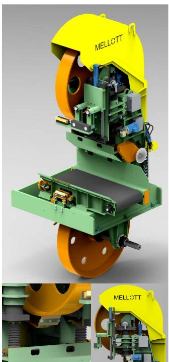
Top wheel scraper tilts and moves up and down with the top wheel. Column support tubes are 8" diameter and nitride coated
