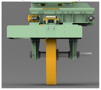
Lower wheel uses rail car bearings. Bearing housings are keyed and bolted. All alignment adjustments are made at the top wheel
