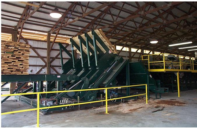
Optional conveyors include: Infeed decks, outfeed conveyors, stick removal conveyors and stick stacking systems. Combined, these conveyors make a reliable, heavy duty tilt hoist system.
