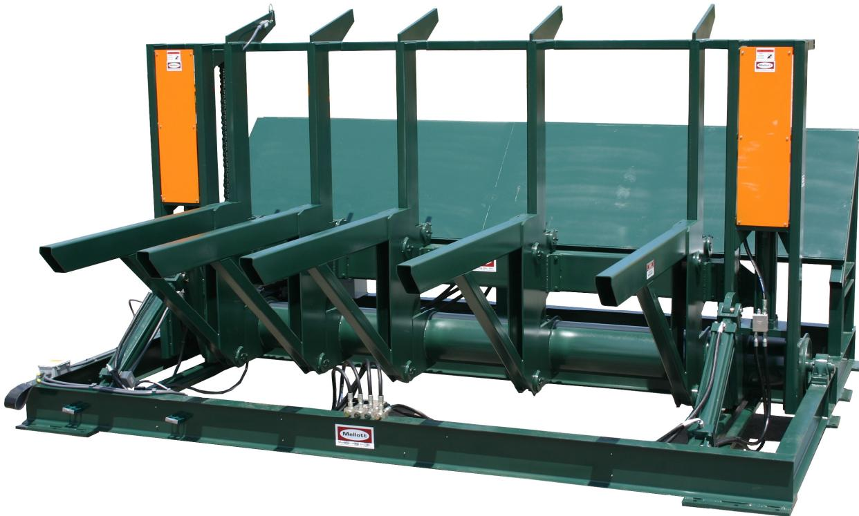
The Mellott 15 Ton Tilt Hoist is designed to unstack stickered packages of lumber. The standard machine is designed for 72" high x 96" wide x 16' long packages. Different columns and forks are available.
