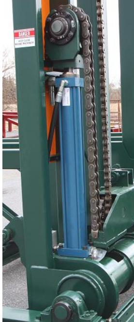
Dual Steel lift cylinders with heavy RC160 roller chain
