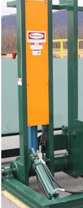
Lift cylinders are guarded to prevent damage to the cylinders and kiln sticks
