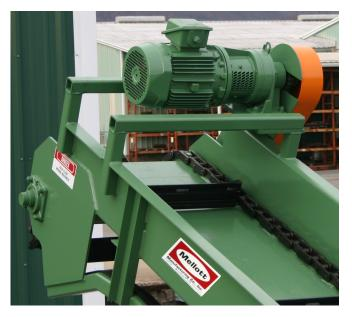
The electric drive is a foot mounted Sumitomo designed for rugged applications.
