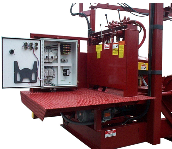
ALL CONTROLS AND MOTOR STARTERS ARE INCLUDED AND PRE-WIRED
