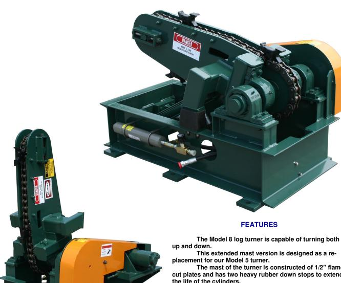
The Model 8 is pivoted on a 2 7/16" diameter shaft with double row spherical roller bearings with cast • steel housings.
