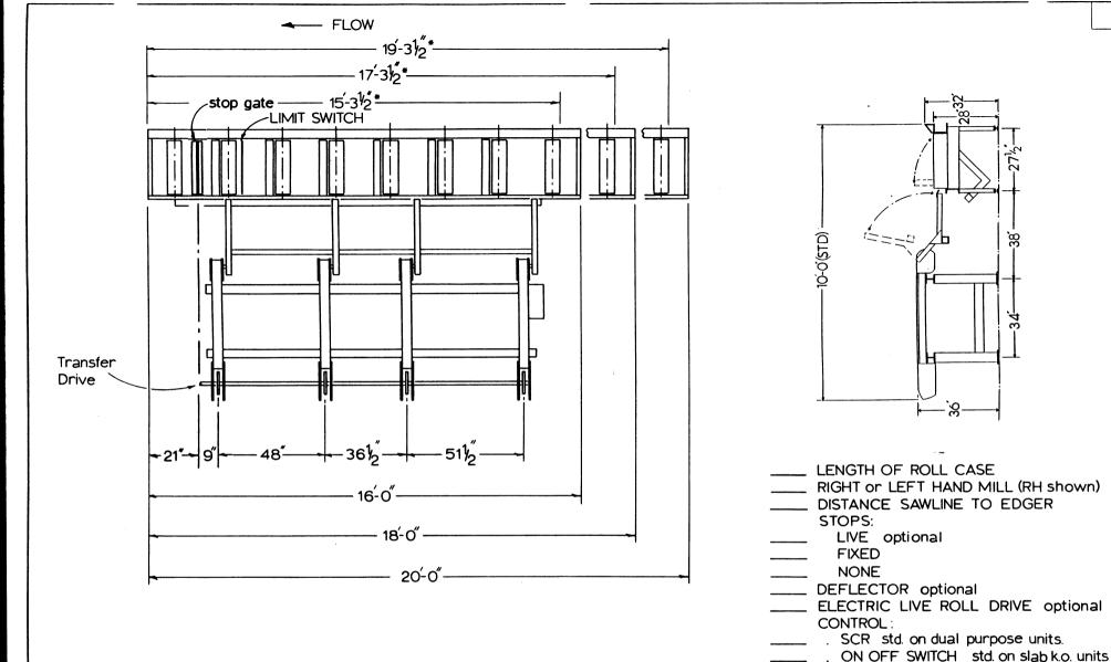
\* Length of roll case when located downstream from belted section with drop out space or drop belt.
